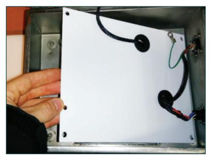
5: Lift plate to access circuit board
