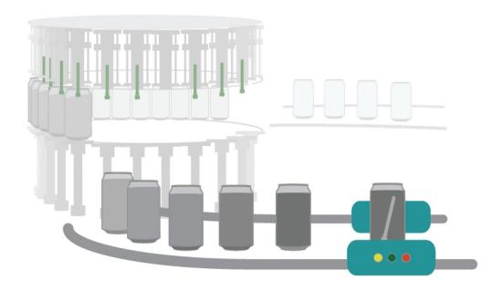
The VTDS uses patented state of the art technology to The system consists of two sense the presences of a traceable vent tube in a can. The standard Enrpo VTDS provides the filling machine owner / operator with both visual indications (as discussed above) as well as discrete 24VDC output signal whenever a vent tube malfunction occurs. The VTDS requires the use of Enrpo's patented Traceable Vent Tubes in order to reliably and accurately sense the presence of a traceable vent tube.
