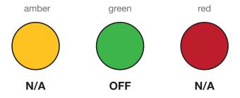
Amber = Vent Tube Detected - The amber light will illuminate when a traceable vent tube is located
