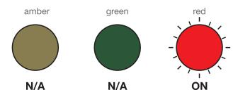
Unit is sensing an Error
