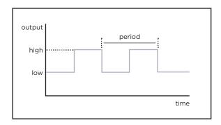
Please contact Enrpo for your specific ideal programming signal output conditions. Maintenance The heartbeat function of the VTDS provides the user a continual 24 VDC system health check. The duty cycle and frequency can be customized to the users specifications.
